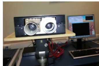
Fig. 1. The proposed device to capture iris image sequences.
